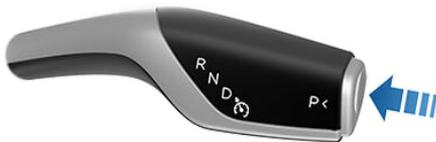
Model Y automatically shifts into Park whenever you connect a charge cable or if two or more of the following conditions are met simultaneously while traveling slower than approximately 1.5 mph (2 km/h):
