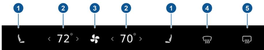
1. Seat heaters operate at three setting levels from 3 (highest) to 1 (lowest). When operating, the associated seat icon displays twisting lines that turn red to indicate the setting level. If equipped with the premium package, rear seats are also equipped with seat heaters (see [Operating Seat Heaters](#) on page 129).
