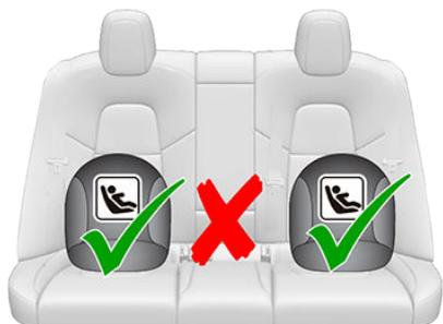
To install a LATCH child safety seat, slide the safety seat latches onto the anchor bars until they click into place. Carefully read and follow the instructions provided by the child safety seat manufacturer.
