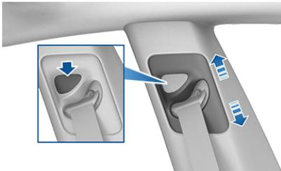
3. Release the button on the shoulder anchor so that it locks into position.
