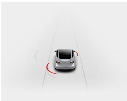
Lane Assist also warns you when a desired lane departure is not appropriate. When you engage the turn signal and a vehicle or object is detected in the adjacent lane you are planning to move into, the touchscreen displays a red lane line to indicate that a vehicle or object is detected. When the vehicle or object is no longer detected, the lane line returns to normal.
