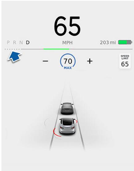
While this alert is present, the deceleration rate of the vehicle due to regenerative braking will be reduced and more brake pedal application will be required to slow the vehicle (similar to what is needed in a gas-powered, non-electric, vehicle).
