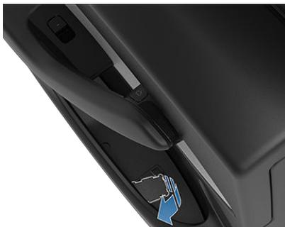
3. Pull the mechanical release cable (foam block) to release the door latch.
