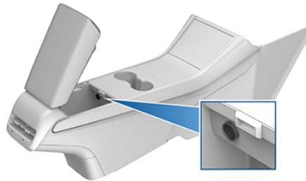
The power socket is suitable for accessories requiring up to 12A continuous draw (16A peak).
