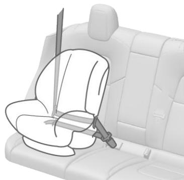
2. Allow the seat belt to retract, and remove all slack in the seat belt while firmly pushing the child safety seat into the Model Y seat.
