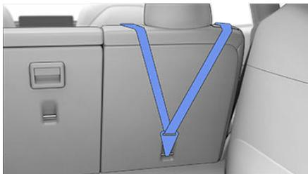
For dual-strap tethers, position a strap on each side of the head support.
