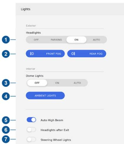
1. Exterior lights (headlights, tail lights, side marker lights, parking lights, and license plate lights) are set to **AUTO** each time you start Model Y. When set to **AUTO**, exterior lights automatically turn on when driving in low lighting conditions. If you change to a different setting, lights always revert to **AUTO** on your next drive.
