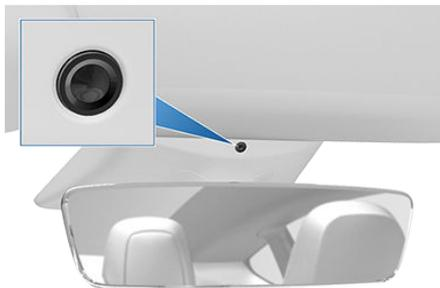
Keep the camera lens clean, and free of obstructions. Remove any buildup of dirt or dust by occasionally wiping the camera lens with a soft damp cloth.
