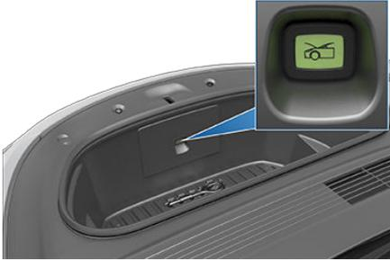
Press the interior release button to open the front trunk, then push up on the hood.
