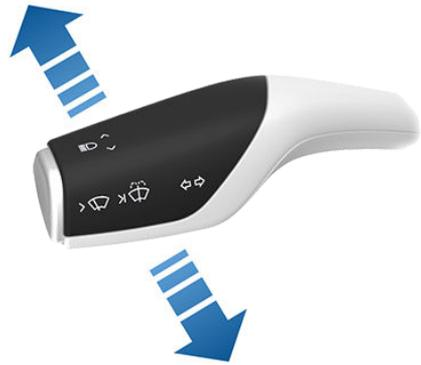
The high beam headlights can automatically switch to low beam when there is light detected in front of Model Y (for example, from an oncoming vehicle). To turn this feature on or off, touch **Controls > Lights > Auto High Beam**.
