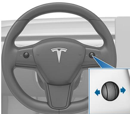
You can also display and adjust the setting for the following distance on the touchscreen at any time, even when Traffic-Aware Cruise Control is not active. Touch **Controls** > **Autopilot** > **Cruise Follow Distance**, then adjust the following distance by touching plus (+) or minus (-).
