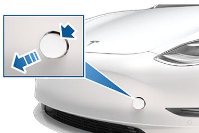
3. Fully insert the tow eye into the opening, then turn it **counter-clockwise** until securely fastened.
