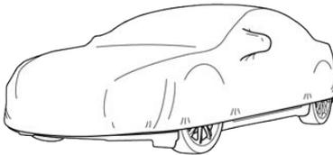
**⚠ Caution:** Use only a Tesla-approved car cover when Model Y is plugged in. Using a non-Tesla car cover can prevent the Battery from being adequately cooled during charging.
