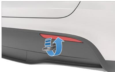
4. Attach the winch cable to the tow eye.
