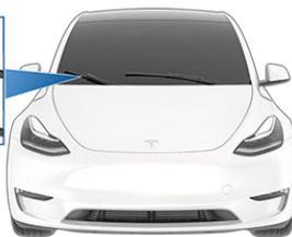
6. Align the new wiper blade on the wiper arm and slide it toward the end of the wiper arm until it locks into place.
