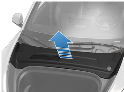
3. If checking the Battery coolant, remove the cabin intake trim panel by pulling it upwards to release the clips that hold it in place.
