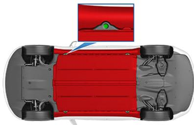
3. Adjust the height and position of the lift arm pads to ensure that they are correctly located.
