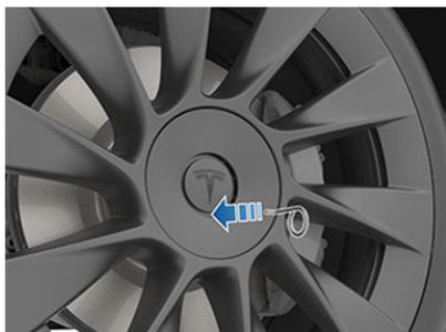
2. Twist the lug nut cover tool so that the end of the curved part is facing away from the Tesla "T".
