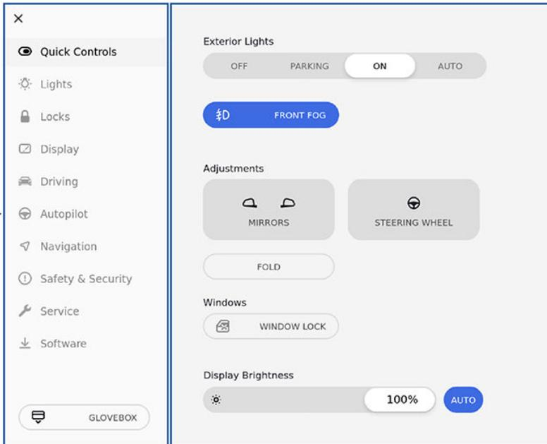
1. Control tabs and open glovebox. When you select an item from the list of tabs, its associated controls and options display in the main viewing area.
