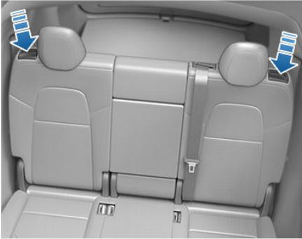
To maximize cargo space, each second row seat back can be folded fully forward to lay flat. While pulling and holding the handle, push the corresponding seat back fully forward.
