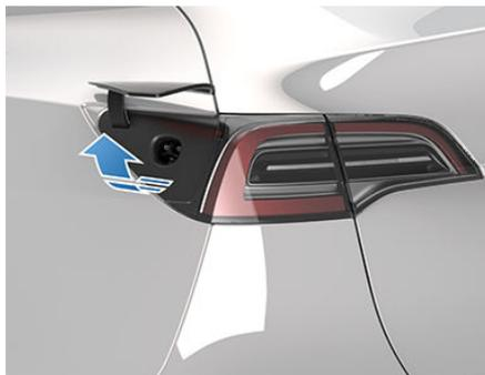
**Note:** The Tesla "T" lights up white when you open the charge port door. If you do not insert a charge cable into the charge port within a few minutes after opening the charge port door, the charge port door closes. If this happens, use the touchscreen to open the charge port door again.
