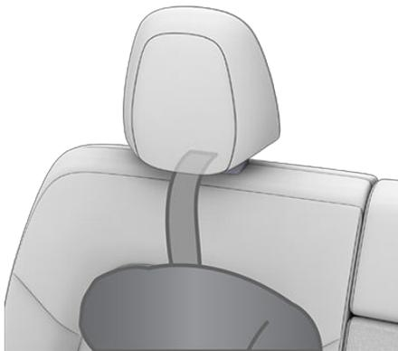
For a single-strap tether at the center seating position, raise the head support (see [Raising/Lowering the Rear Center Head Support](#) on page 30) and run the strap under the head support.
