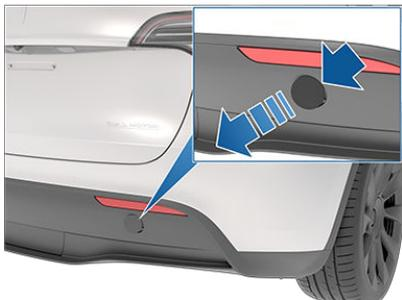
3. Fully insert the tow eye into the opening, then turn it **counter-clockwise** until securely fastened.
