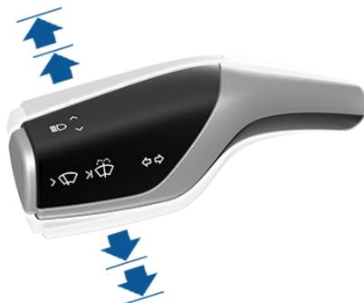
The turn signals stop operating when canceled by the steering wheel, by moving the lever in the opposite direction, or lightly pushing the lever in the same direction once more.
