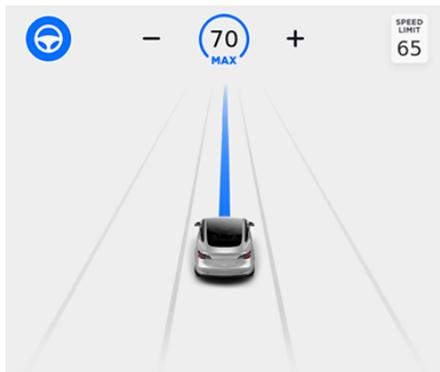
When Navigate on Autopilot is active and you approach an off-ramp or freeway interchange along your navigation route, the appropriate turn signal engages and Autosteer maneuvers Model Y onto the off-ramp or interchange.
