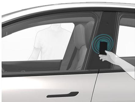
Once inside, power up Model Y by pressing the brake pedal within thirty seconds of scanning the key card (see [Starting and Powering Off](#) on page 56). If you wait longer than thirty seconds, you must re-authenticate by placing the key card near the card reader located behind the cup holders on the center console. When your key card is detected, your 30 second authentication period restarts.
