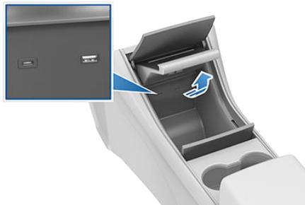
Two additional USB-C ports are located in the rear of the center console. Passengers in the rear seats can use these ports to charge their USB-connected devices. Devices connected to the rear USB ports do not communicate with the vehicle.
