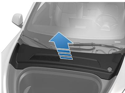
3. Remove the cabin intake trim panel by pulling it upwards to release the trim clips that hold it in place.
