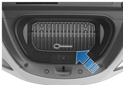
2. Release the front tow eye cover by pressing firmly on its top right perimeter until it pivots inward, then gently pulling the raised section toward you.
