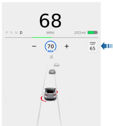
In situations where Model Y is unable to determine a speed limit, or if Speed Assist is uncertain that an acquired speed limit is accurate, the touchscreen may not display a speed limit sign and warnings do not take effect.
