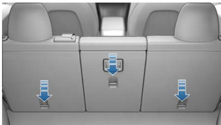
Make sure the hook is fully seated on the anchor point.
