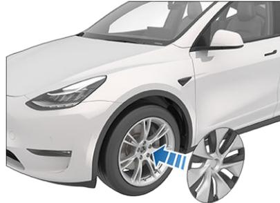
2. Push firmly around the perimeter of the aero cover until it fully snaps into place.
