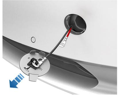
4. Connect the 12V power supply's red positive (+) cable to the red positive (+) terminal.
