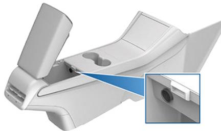
The power socket is suitable for accessories requiring up to 12A continuous draw (16A peak).
