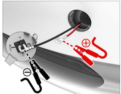
**Note:** Applying external 12V power to these terminals only releases the hood latches. You cannot charge the 12V battery using these terminals.
