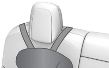
For a single-strap tether at an outboard seating positions, raise the head support (see [Raising/Lowering the Outer Rear Seat Head Supports](#) on page 30) and run the strap under the head support.
